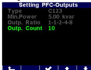
After entering the tool, in the window you can set the output type and minimum (nominal) output reactive power ( $O_{MIN}$ ), then select one of predefined output ratio and, finally, specify total number of outputs.
