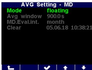
Parameters determining maximum demand processing can be set in the **Setting – AVG – MD** screen. As default, *the floating window averaging method* is set.
