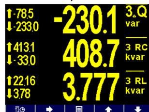
For compensation reactive power capacity assessment, registered minimum values of both reserves are decisive (data with a prefix ↓). On the left example above, registered minimum of three-phase
