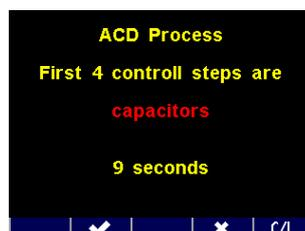
During following 10 seconds, you can either cancel the start command with the button or to skip the message timeout with the button to start the CT test immediately. Or you can simply let the timeout to expire and then the ACD starts.
