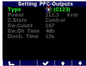
In the first two rows, there are shown again the output type and its nominal three-phase reactive power. To set any of these parameters correctly you must specify the output type first : scroll to the output type and push the button. A pop-up menu with assortment of available output types appears and now you can selected desired one. After confirmation with the , new output type is assigned. Now you can modify the output reactive power.
