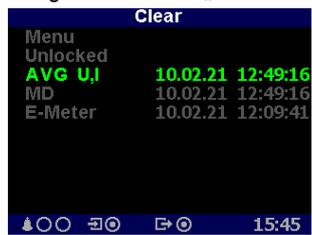
The *Unlocked* informs that clearing of the quantities is not locked now.
