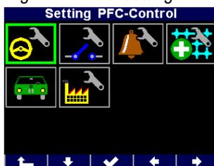
The complete PFC setting consists of a series of parameters arranged into four groups : **the PFC Control**, **the PFC Outputs**, **the PFC Alarms** and **the PFC Grid Support** . Next two options in the menu are **the Control <-> Manual** state toggle and **the PFC Factory Setting** utility.
