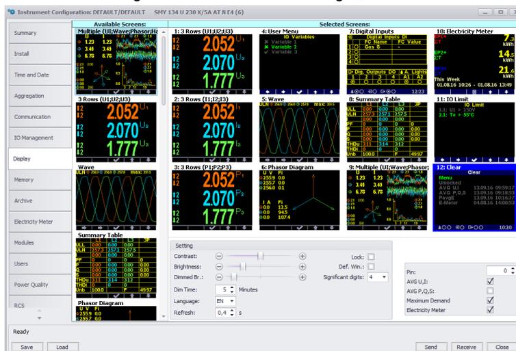
Check the quantity groups that you want to allow clearing from the screen – at the example above there are *AVG U/I*, *Maximum Demand* and *Electricity Meter* groups. Now send the setting into the instrument.
