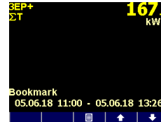
Fig. 4.30 : Custom Electricity Meter Screen with Bookmark
