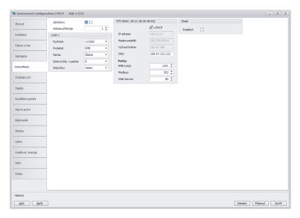
Figure 16: ENVIS.Daq — setting of communication line parameters.
