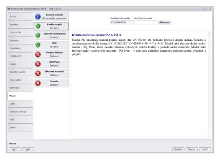
Figure 21: ENVIS. Daq — Activation of special firmware modules.
