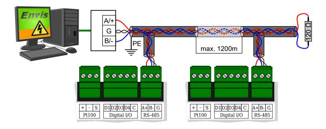
Figure 9: Connection of RS-485 communication lines to BCPM 233.012 devices BCPM 233.012.
