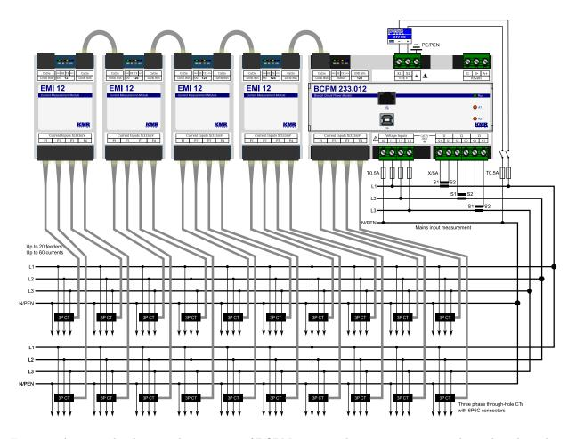
Figure 8: An example of a typical connection of BCPM 233.012 when measuring many three-phase branches. The device is extended by 4 pieces of EMI 12 modules connected via local bus.
