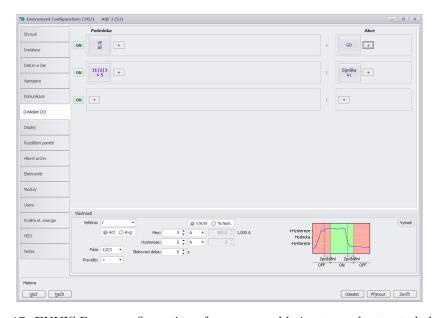
$Figure \ 17: \ ENVIS. Daq \ \hbox{--} configuration of programmable inputs and outputs behavior. }$
