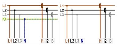
(b) Connection types of devices in LV networks (direct connection).
